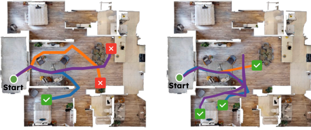
(a) 3D-Mem trajectories on a representative MP3D scene. Under episodic evaluation, the agent re-explores from scratch for each query, answering only 1/3 correctly. Persistent 3D memory enables more direct navigation and correct answers for all 3 questions.
